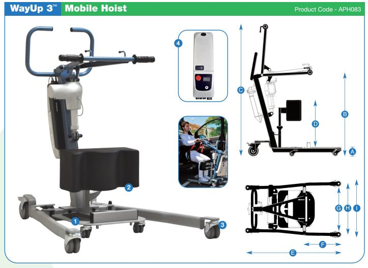
The **WayUp 3** mobile hoist has been designed as a compact stand and assist aid. The electric **WayUp 3** can be used for transfer stand and assist, featuring a multi-adjustable lift boom with an ergonomic lift angle designed to minimise shear and friction when lifting. Simple electric adjustment helps to manoeuvre the stand assist into small or confined spaces. The base legs can be electrically adjusted for added stability.
